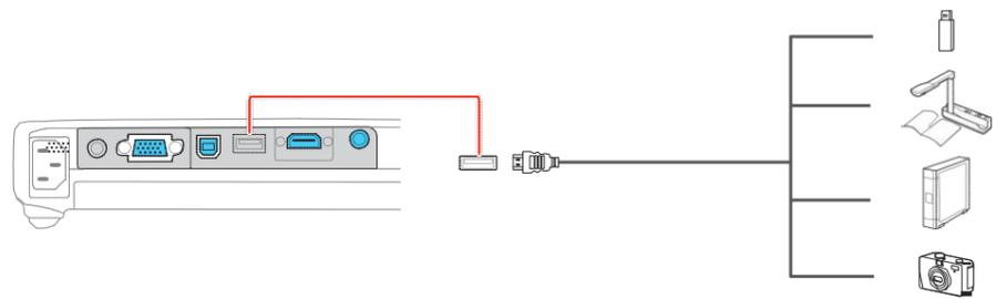
If you connect a digital camera, USB flash drive, or USB storage device, you can use the projector's Slideshow feature to project images. See the online *User's Guide* for details.
