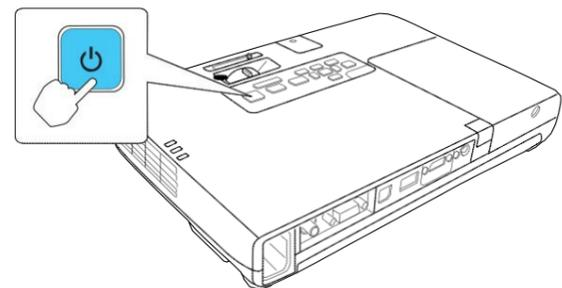
**Note:** To shut down the projector, press the power button twice, then unplug it. You don't have to wait for the projector to cool down.
